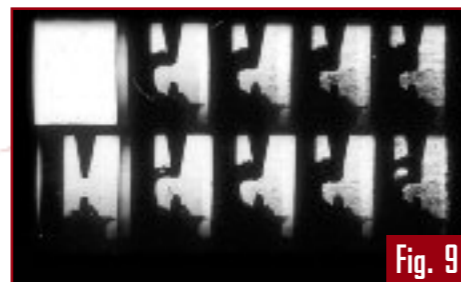
High-speed recording of an irregular spark discharge (frame rate: 2 \times 10^6 frames per second). The propagation of a bent, hose-shaped plasma bubble can be recognized. This is caused by a spark that does not take the direct path between the electrode peaks but attaches to the side of the electrodes. Precise focusing through a rotation ellipsoid is no longer guaranteed because of the deviation from the spherical geometry.
