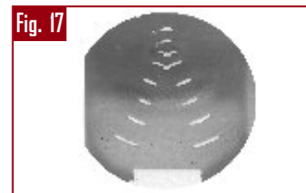
Schlieren photograph of the fronts of successive waves on the way from the reflector to the treatment zone.
