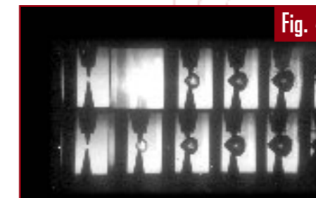
High-speed recording of a spark discharge (Frame rate: 2 x 10 6 frames per second). The spark ignition takes place in frame 2 of the upper row. A plasma bubble subsequently forms. A shock wave cannot be detected yet. It has already detached itself between the second frame of the first row and the second frame of the second row.
